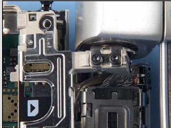
26. ...and gently separate the Upper Block from the Lower parts.
