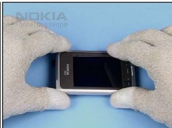
6. Aligne the FLIP A-COVER with the FLIP FRAME ASSY...
