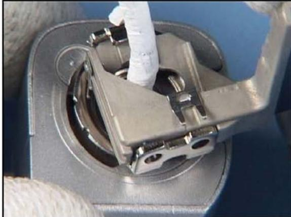
14. Position the GRIP INNER FRAME onto the HINGE ASSEMBLY.
