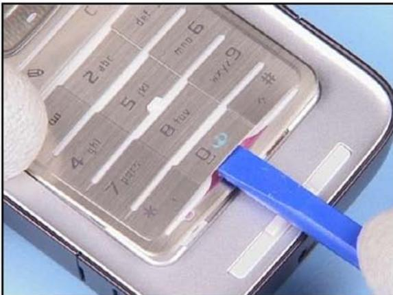
3. Optionally the KEYMAT can be removed now. Lift the KEYMAT with the SS-93 as shown.
