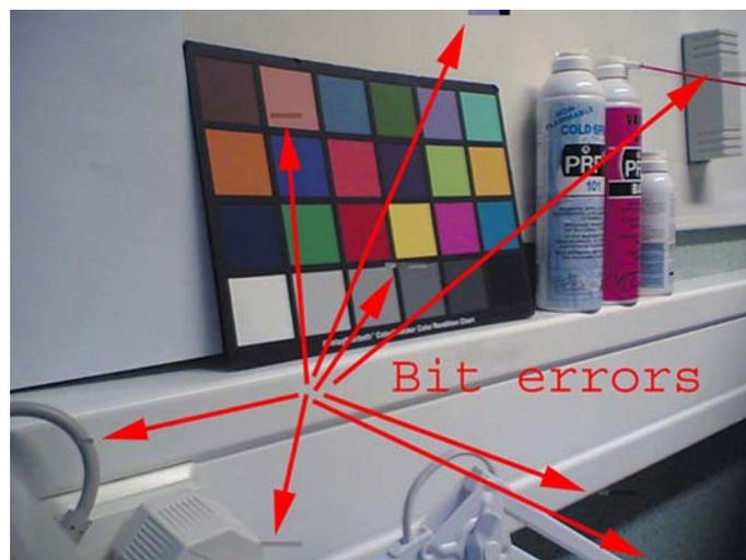
Figure 74 Bit errors caused by JPEG compression
