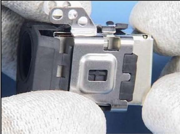
37. Insert the CAMERA MODULE into the FRAME.
