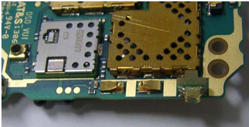
**Figure 108 Bluetooth/WLAN contact**
