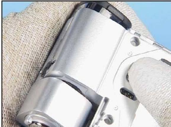
18. Unlock the last two snaps on the hinge side and remove the GRIP B-COVER.
