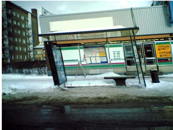
**Figure 62** Near objects get skewed when taking images from a moving vehicle
