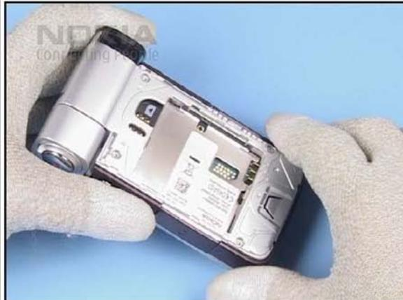
2. Remove the battery if inserted.
