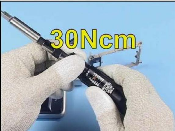
15. Set torque driver to the correct torque.
