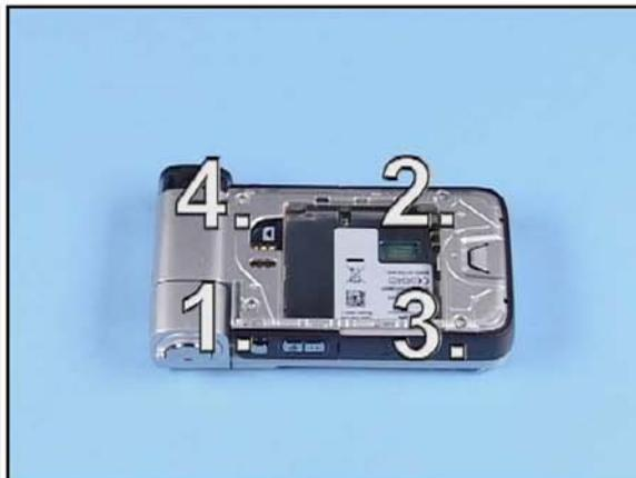
8. Undo the four Torx Plus size 6 screws in the order shown.
