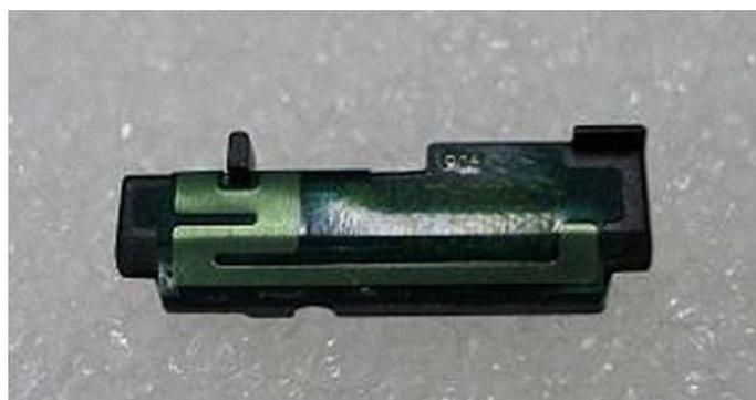
**Figure 41 Bluetooth antenna module**
