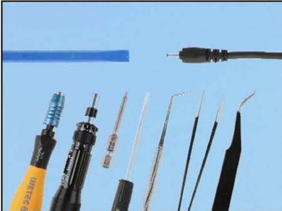
1. Needed Tools: a Torx driver, a torque driver, a Torx Plus size 6 bit, a flat bladed screwdriver, a dental pick, metal tweezers, angled tweezers, the SS-93 and the DC-plug.
