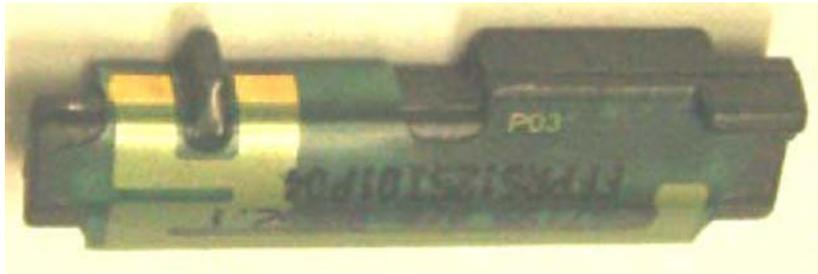
**Figure 107 Bluetooth/WLAN Antenna**
